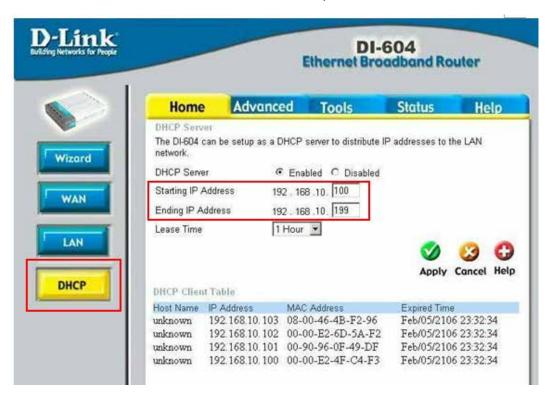
Here are "Starting IP Address" and "Ending IP Address", they are from 192.168.10.100 to 192.168.10.199.
